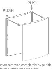
cover removes completely by pushing down buttons on both sides
